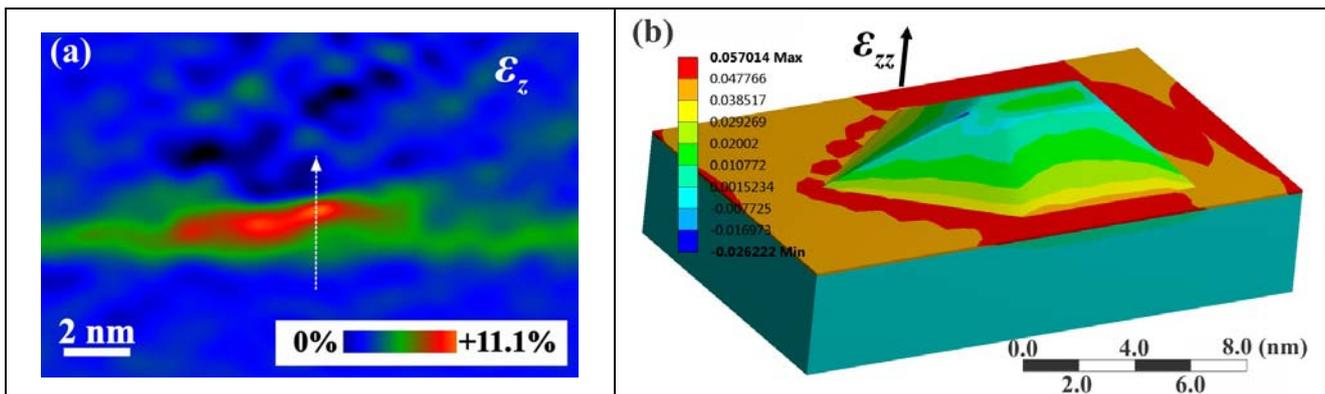
Fig. 1. (a) 2-D GPA strain map along the growth direction, illustrating the gradual increase of the  $\epsilon_z$  strain inside an InAs QD with the GaAs lattice taken as the unstrained reference. (b) 3-D FEM simulated  $\epsilon_{zz}$  elastic strain in an InAs QD model, showing gradual relaxation from the base toward the apex of the QD.
